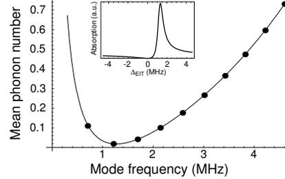
Figure 4. Mean phonon number (black dots) of the axial modes of a 10-ion string *vs* the mode frequencies, after EIT-cooling has been applied to the level scheme of Figs. 2a,2b. Here, the c.o.m. axial trap frequency is assumed to be 0.7 MHz, while  $\Omega_\sigma = 20$  MHz,  $\Omega_\pi = 0.5$  MHz, and  $\Delta_\sigma = \Delta_\pi = 75$  MHz, giving a light shift  $\delta \sim 1.3$  MHz (see inset).
