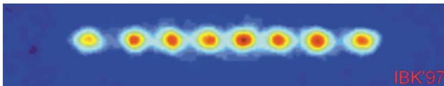
**Counting qubits: a string of ions representing a 'quantum byte' in an ion-trap quantum computer. Here all are in state '0'; exciting any one would cause loss of fluorescence at the corresponding position.**
