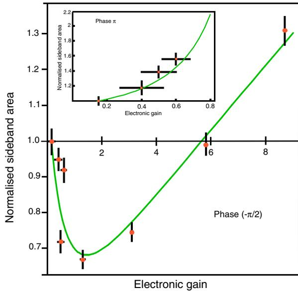
FIG. 3 (color online). Steady-state energy of the cooled oscillator: measured sideband area, normalized to the value without feedback, versus gain of the feedback loop, for  $(-\pi/2)$  (main plot) and  $\pi$  (inset) feedback phase. The curves are the model calculations. The gain axis is scaled to the experimental values of the electronic gain.
